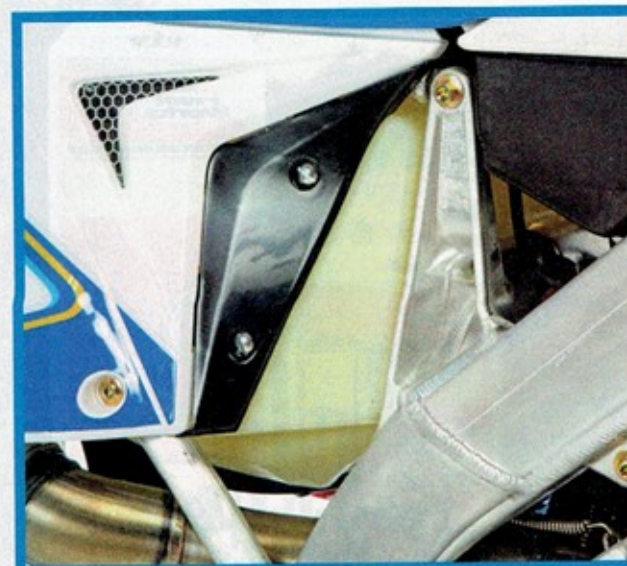
The gas tank is made from translucent plastic that allows you to tell how much fuel is left at a casual glance.
