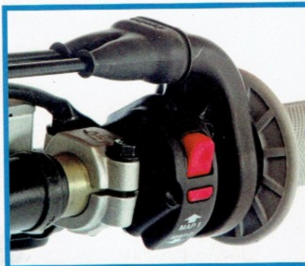
Press the top red button for the aggressive map and the bottom red button for the mellow map.
