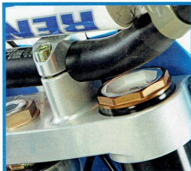
Look ma, no air valves. TM's Kayaba SSS forks need a little help in the mid-stroke. We lower the oil height by 10cc.
