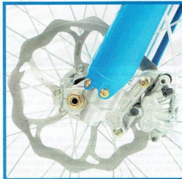
Imagine a KTM Brembo front brake mated to a 270mm rotor and you have an idea of how well the TM stops.
